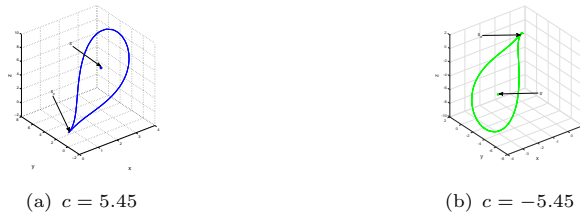
Fig. 3. Phase portraits of system (2.2) with (a, b) = (2, 3) , (a) c = 5.45 , (x_0, y_0, z_0) = (1.3, 1.6, 1.6) \times 1e-4 , (b) c = -5.45 and (x_0, y_0, z_0) = -(1.3, 1.6, 1.6) \times 1e-4 . The figures illustrate that system (2.2) has a homoclinic trajectory to S_0 when (a, b, c) \in W_{212}^3 .
