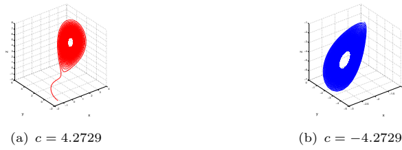
Fig. 1. Phase portraits of system (2.2) with (a, b) = (2, 3) and different values of parameter c .
