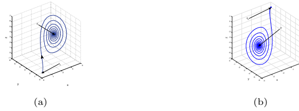
Fig. 6. Phase portraits of system (2.2) with (a) (a, c, b) = (2, 4, 4) , (x_0, y_0, z_0) = (1.3, 1.6, 1.6) \times 1e - 4 , (b) (a, c, b) = (2, -4, 4) , (x_0, y_0, z_0) = -(1.3, 1.6, 1.6) \times 1e - 4 . These figures illustrate that system (2.2) has one and only one heteroclinic trajectory to S_0 and S' when (a, b, c) \in W_{211} .
