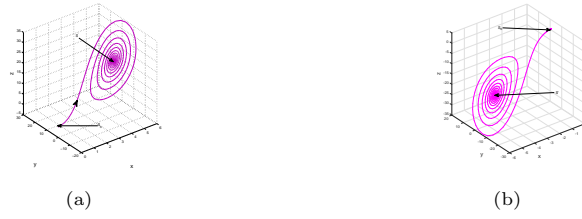
Fig. 4. Phase portraits of system (2.2) with (a) (a, c, b) = (2, 19, 6) , (x_0, y_0, z_0) = (1.3, 1.6, 1.6) \times 1e-4 , (b) (a, c, b) = (2, -19, 6) , (x_0, y_0, z_0) = -(1.3, 1.6, 1.6) \times 1e-4 . These figures illustrate that system (2.2) has one and only one heteroclinic trajectory to S_0 and S' when (a, b, c) \in W_{211} .
