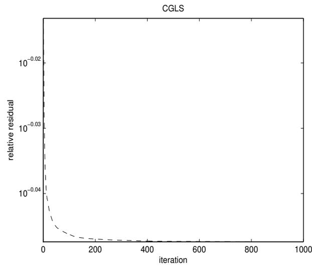
**Figure 1.**  $\|A^T r\|_2 / \|A^T b\|_2$  vs. iterations ( $m = 5000$ ,  $n = 1000$ , density=0.01, condition number= $10^6$ ,  $r = 50$ )
