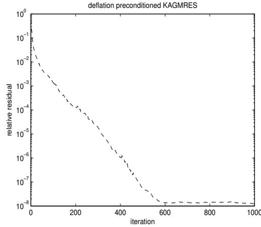
**Figure 5.**  $\|A^T r\|_2 / \|A^T b\|_2$  vs. iterations ( $m = 5000$ ,  $n = 1000$ , density=0.01, condition number= $10^8$ ,  $r = 50$ )
