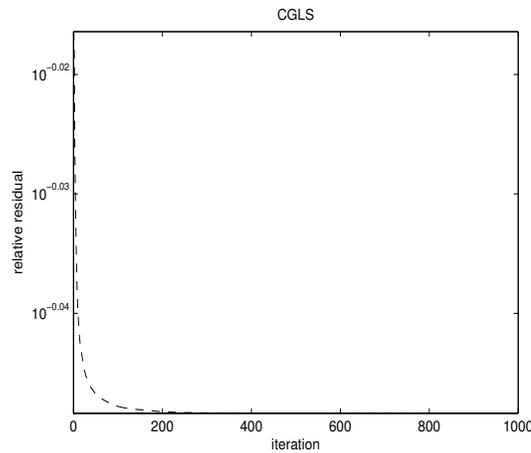
**Figure 4.**  $\|A^T r\|_2 / \|A^T b\|_2$  vs. iterations ( $m = 5000$ ,  $n = 1000$ , density=0.01, condition number= $10^8$ ,  $r = 50$ )
