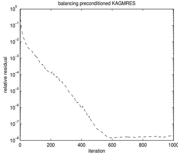
**Figure 6.**  $\|A^T r\|_2 / \|A^T b\|_2$  vs. iterations ( $m = 5000$ ,  $n = 1000$ , density=0.01, condition number= $10^8$ ,  $r = 50$ )
