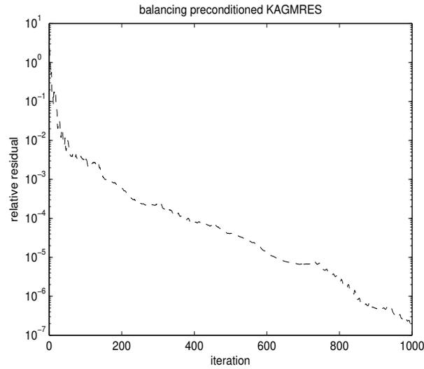
**Figure 3.**  $\|A^T r\|_2 / \|A^T b\|_2$  vs. iterations ( $m = 5000$ ,  $n = 1000$ , density=0.01, condition number= $10^6$ ,  $r = 50$ )
