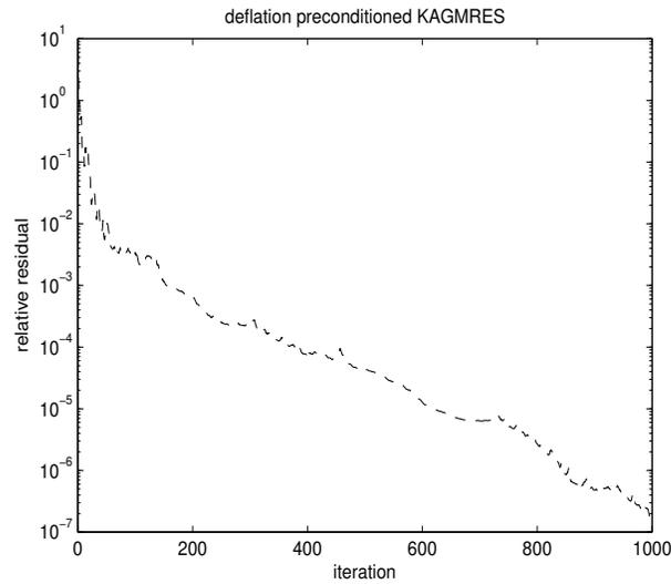
**Figure 2.**  $\|A^T r\|_2 / \|A^T b\|_2$  vs. iterations ( $m = 5000$ ,  $n = 1000$ , density=0.01, condition number= $10^6$ ,  $r = 50$ )
