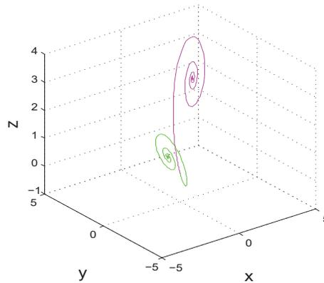
**Fig. 6.** Phase portrait of system (1.1) when  $(a, b, d, f, g) = (3, 12, 2, 1, 1)$  and  $(x_0, y_0, z_0) = (\pm 3.14 \times 1e - 4, \pm 1.618 \times 1e - 4, \pm 2.718 \times 1e - 4)$ . This figure illustrates that system (1.1) has two heteroclinic orbits for  $bg = 2a(f + g)$  and  $a > d > 0$ .
