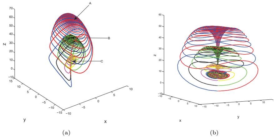
**Figure 5.** Phase portraits of system (1.1) when  $(a, d, f, g) = (9, 8, -2, 4)$ , (a)  $b = 0$ , (b)  $b = 0.1$ , and the initial values  $(x_0, y_0, z_0) = (\pm 1.618 \times 1e - 3, \pm 1.618 \times 1e - 3, z)$ , (A)  $z = 5$ , (B)  $z = 0$ , (C)  $z = -5$ . These figures illustrate that system (1.1) has infinite many singularly degenerate heteroclinic cycles and corresponding chaotic attractors.
