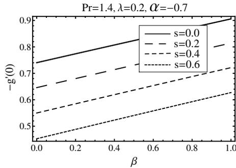
**Figure 9.** Effect of source/sink on heat transfer rate (PST case).
