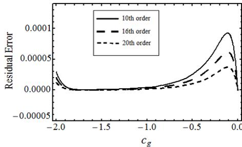
**Figure 3.** Exact residual error for the function  $G(\eta)$ .
