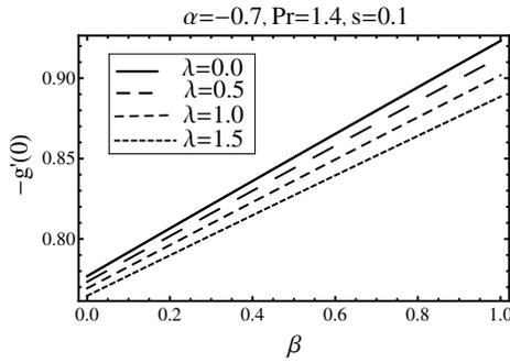
**Figure 10.** Effect of viscoelastic parameter on heat transfer rate (PST case).
