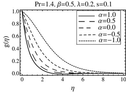
**Figure 11.** Effect of mass transfer parameter on temperature profiles (PST case).
