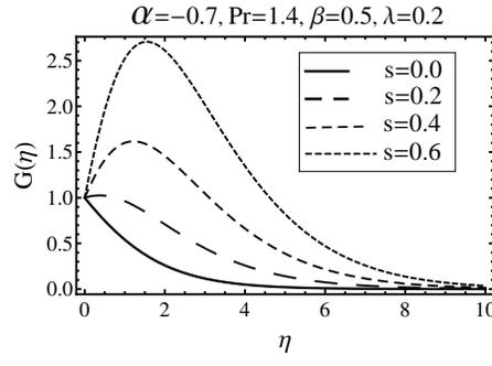
**Figure 8.** Effect of source/sink on temperature profiles (PHF case).
