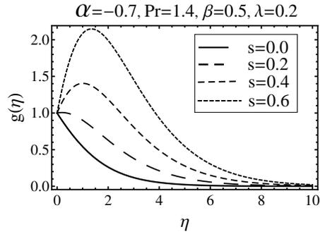
**Figure 7.** Effect of source/sink on temperature profiles (PST case).
