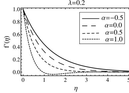
**Figure 6.** Effect of mass transfer (injection) on velocity profiles.
