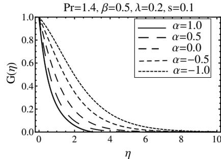
**Figure 12.** Effect of mass transfer parameter on temperature profiles (PHF case).
